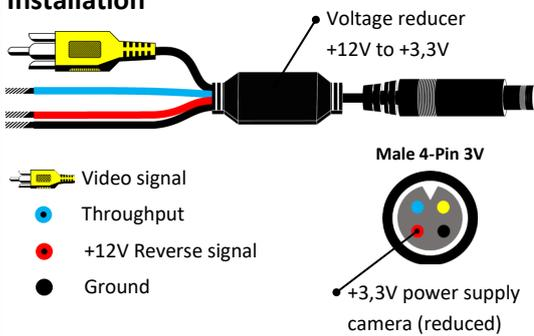
**Note:** If the camera is powered by reverse gear lamp signal, we recommend to install a relay between the power supply of the reverse signal and the power supply of the camera, to ensure a stable and uninterrupted power supply and to avoid errors in the vehicle computer.
