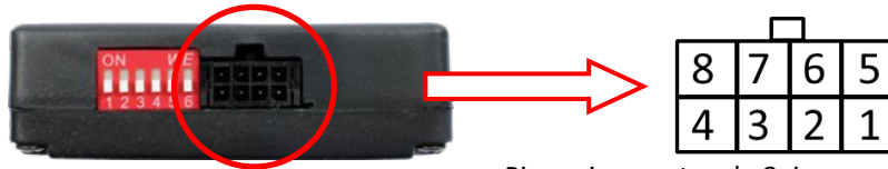
Pin-assignment male 8pin connector of TV-500
